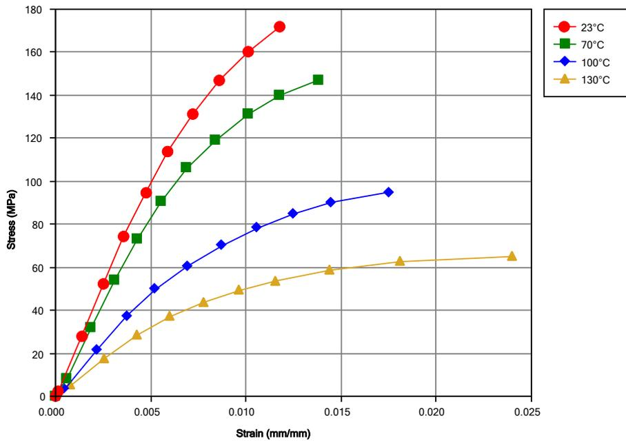
Secant Modulus vs. Strain (ISO 11403-1)
