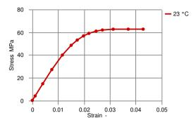
dry sample is dry as molded 23°C yield at 0.03132 strain, 62.627 stress Poisson ratio used: 0.38
